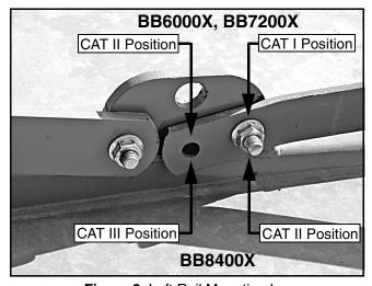
Figure 3. Left Rail Mounting Lug
